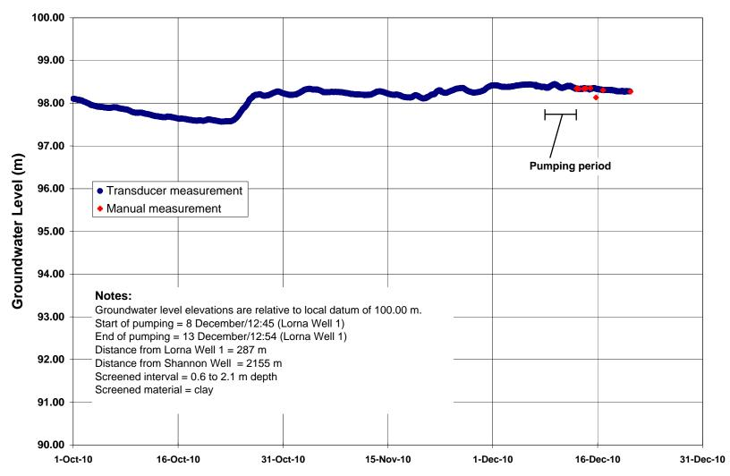
Appendix C-5: CEG Pumping Test, 2010 Hydrograph of Monitoring Well MW6D
