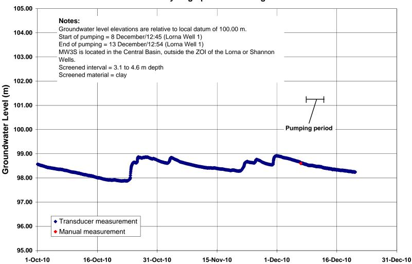
Appendix C-5: CEG Pumping Test, 2010 Hydrograph of Monitoring Well MW4D
